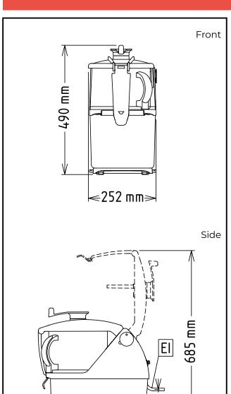
Electric Supply voltage: 600431 (DTRK45Y) 200-240 V/1N ph/50/60 Hz Electrical power max.: 1 kW **Total Watts:** 1 kW Capacity: Performance (up to): 550 kg/hour Capacity: 4.5 litres Key Information: External dimensions, 252 mm Width: External dimensions, Depth: 485 mm External dimensions, Height:
